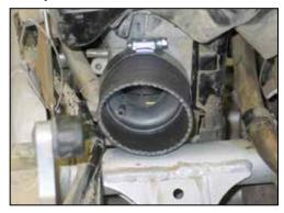
9. Install silicone hose (08405) onto the carburetor inlet and secure with provided hose clamp.
