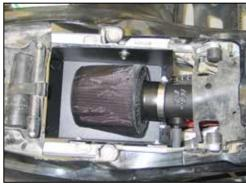
17. Install the K&N<sup>®</sup> air filter assembly onto the intake tube and secure with the provided hose clamp.
