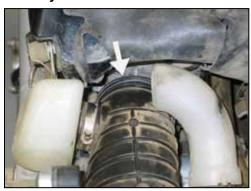
5. Loosen the hose clamp that secures the intake tube to the carburetor intake.
