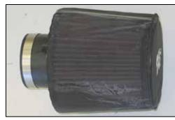
16. Install the K&N® Drycharger® onto the K&N® air filter as shown.
