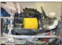
7. Remove the air box assembly from the vehicle as shown.
