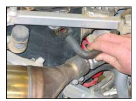
4. Remove the crank case vent hose from the air box.
