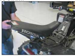
1. Turn off the ignition, unlatch and remove seat and then disconnect the negative battery cable.
