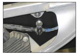
12. Using the factory clip and hardware provided secure the wiring harness to the air box as shown.
