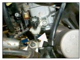
8. Remove the float bowl plug to drain fuel from the carburetor and gain access to the main jet. K&N® recommends replacing the stock main jet with a #170 main jet purchased separately.
